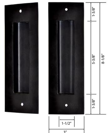
A 1/2" deep pocket must be routed/carved into the door to use the Vista Pull, as the face plate mounts on the door surface
