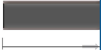
$$\text{Width of Door Slab} - \frac{3}{16} \text{ inch Measurement for BOTH End Caps combined} = \text{Cut Top Track to THIS SIZE}$$
