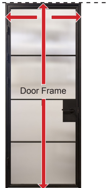
C. Make certain the steel door measurements match up with the doorway measurements.
